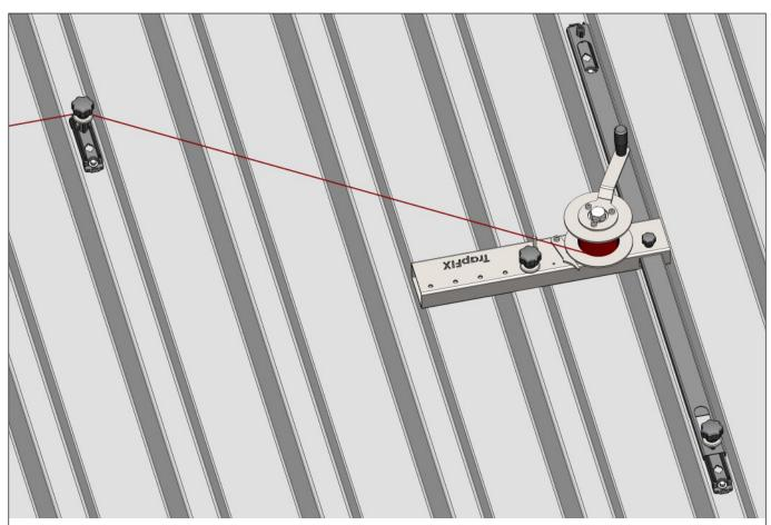
Next, place the 2nd TrapFIX on both sides with the rope as a stop and tension the rope as shown in the picture. Then tighten the rope further and use it as a stop for the top row of TrapFIX. **Caution** Do not shift the rope when placing the TrapFIX.
