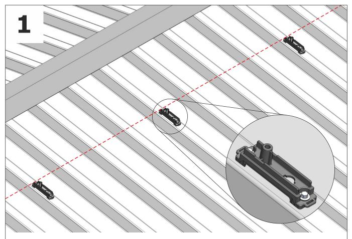
Mount the TrapFIX on the lower or upper roof edge in a straight row using suitable thin sheet metal screws of your choice. The long side of the TrapFix should lie under the modules.
