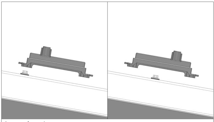
**Bypass roof mounting screws** If the foot of a TrapFIX panel accidentally strikes an existing roof mounting screw, simply rotate the TrapFIX panel 180°. Large calottes may have to be removed.
